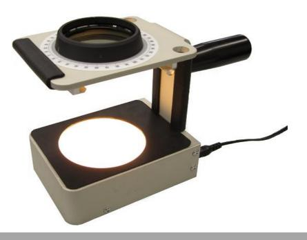
LSM-1000LE visualize a inside stress or birefringence in a transparent material by using polarization technique. It is possible to analyze the optical direction or quantify the retardation relative to inside stress if optional sensitive tint plate or 1/4 wavelength plate is attached to the equipment. It is compact and lightweight. AC adapter is included as standard. Optional battery unit for carrying around and useing is prepared.
