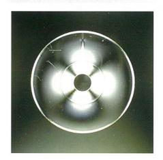
Sample with substantially no strain The whole of a sample appears dark in blackish color similarly to the visual field. Sample with less degree of strain Outer peripheral region of a sample appears in whitish color.
