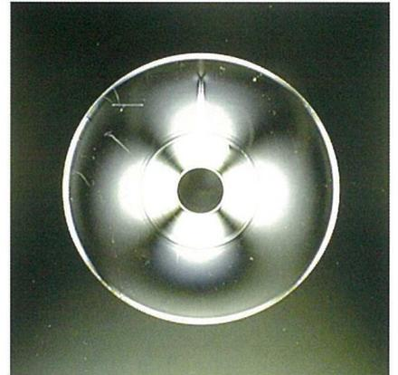
Sample with substantially no strain
