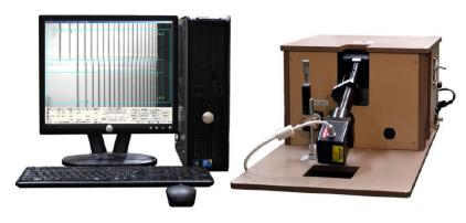
The FSM-6000LE series is developed for measuring the surface stress of glass using a PC.
