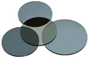
POLAX series consists of various polarizing plates having different properties. Each polarizing plate is made of two pieces of optical glasses and a dichromatic film bonded between them. They are supplied from visible range to infrared range so that they are able to satisfy customer's request.
