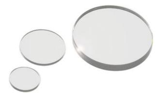
RETAX series consists of various wave plates having different retardation each other. Each wave plate is made of two pieces of optical glasses and a retardation film bonded between them. They are supplied from visible range to infrared range so that they are able to satisfy customer's request. It is possible to select any retardation not just  $1/4 \lambda$ ,  $1/2 \lambda$  and  $1 \lambda$  for the wavelength.
