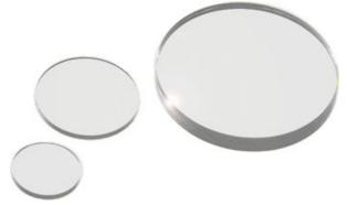
RETAX series consists of various wave plates having different retardation each other. Each wave plate is made of two pieces of optical glasses and a retardation film bonded between them. They are supplied from visible range to infrared range so that they are able to satisfy customer's request. It is possible to select any retardation not just  $1/4 \lambda$ ,  $1/2 \lambda$  and  $1 \lambda$  for the wavelength.
