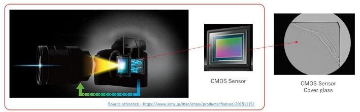
\* If there is striae in the coated or bonded state of the optical components, the image captured in the same way will be "distorted", which will affect the image quality.
