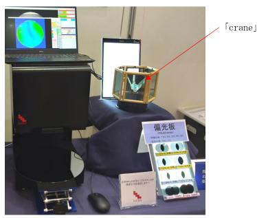
With the fully automatic strain tester LSM-9100WNIR, we were able to receive inquiries and sample measurement requests from visitors by demonstrating the measurement of silicon wafers. Thanks to it, we have gotten some hints to improve our device and information about semiconductor manufacturing process.
